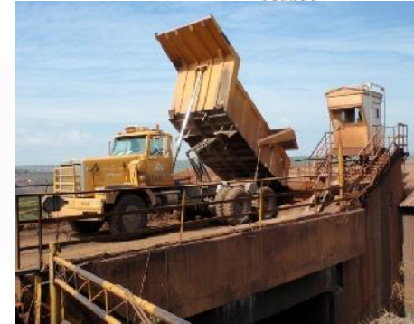
Tipping into Primary Crusher
